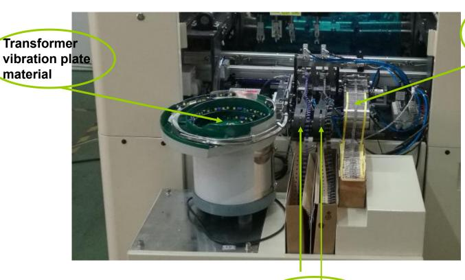
**Resistor feeder** change into capacitor feeder
