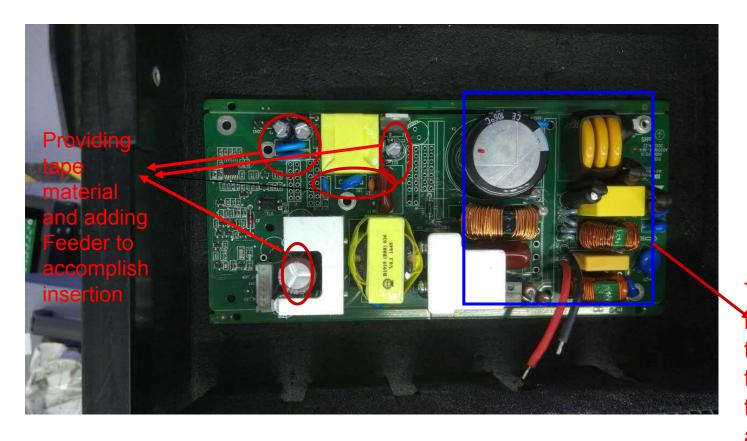
To provide a multi-layer tube with a tube material to achieve automatic feeding insertion
